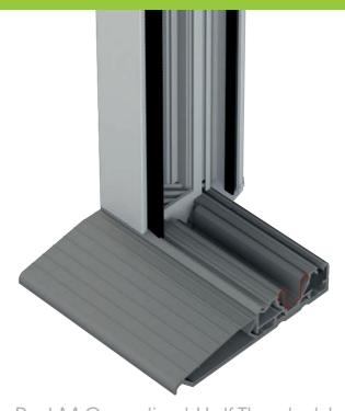
Part M Compliant Half Threshold (Thermally Broken) 26.5mm high
